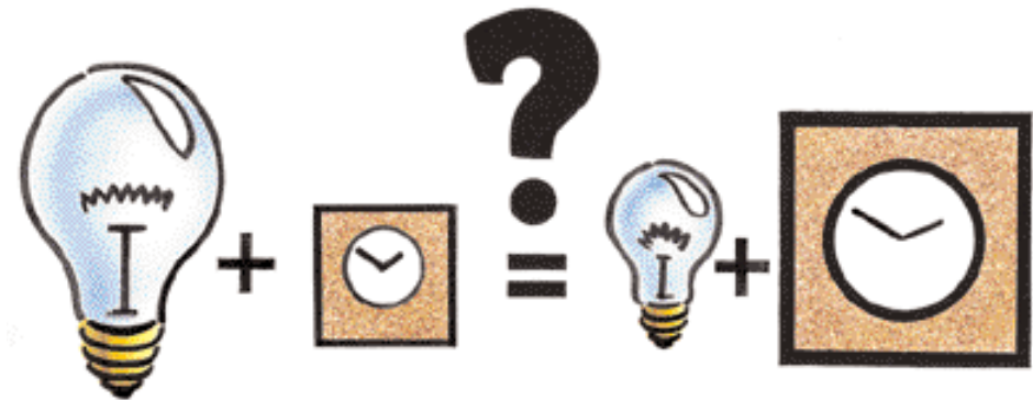
Fig. 5.1.1 A high-power lamp burning for a short time (left) uses the same total amount of energy as a lower-power lamp burning for a longer time (right). However, when considering the effects of timed surgery, equal energies do not achieve equal effects on tissue. The brief, high-power, emission (left) is more effective and more selective in its action than the same amount of energy delivered at low power for a longer time (right).
